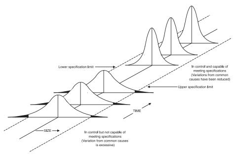
Figure 2.9 From process control to capable process
