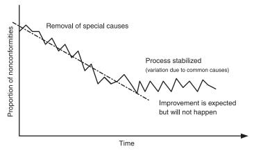
Figure 2.6 Stabilizing processes
