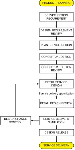
Figure 7.6 Service design process flow
