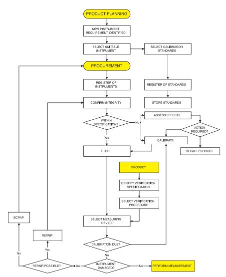
Figure 7.13 Measuring device control process flow
